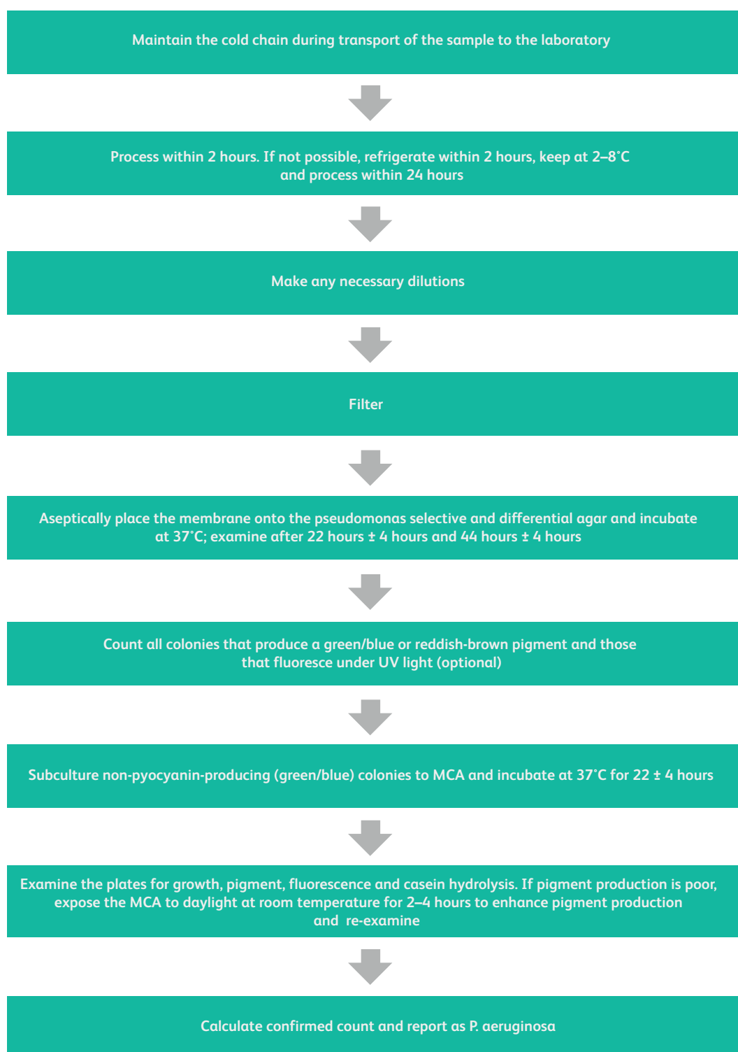
Flowchart showing the processing and enumeration of P. aeruginosa by membrane filtration
