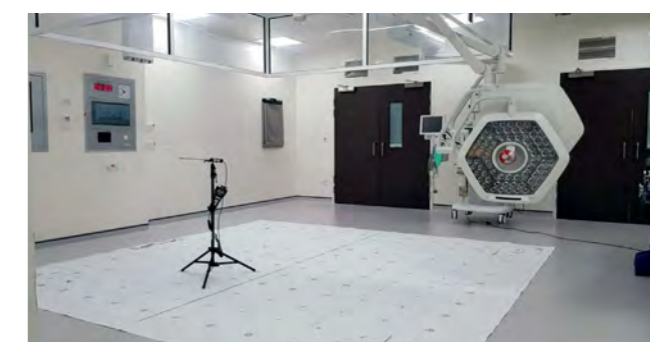
UCV 1m air velocity test set-up
