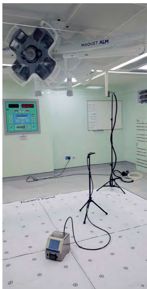
UCV entrainment test setup
