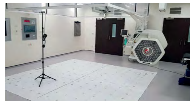
UCV 2m air velocity test set-up
