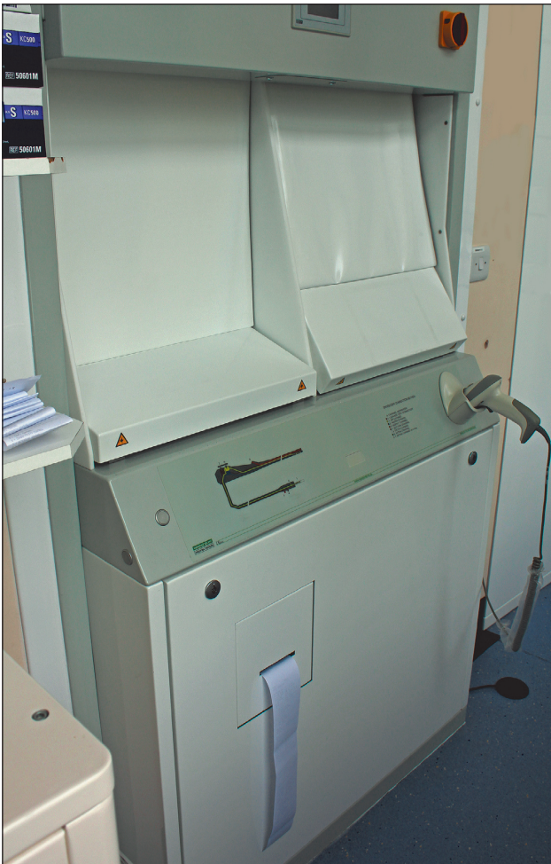
Example of a pass through design AER
