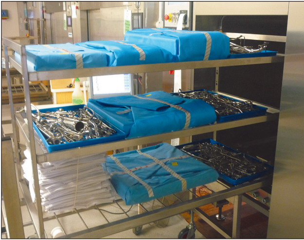
Figure 6 Mixed full load test during validation testing of a sterilizer
