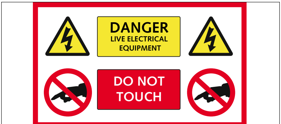
Figure 3 Danger sign (actual size: 200 x 100 x 1.5 mm white plastic)
