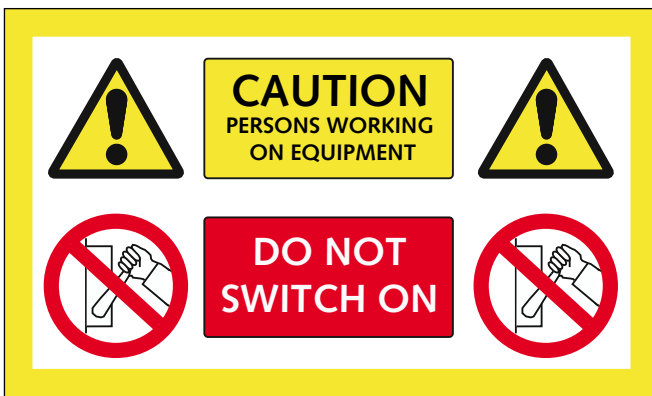
Figure 2 Caution sign (actual size: 200 x 100 x 1.5 mm white plastic)
