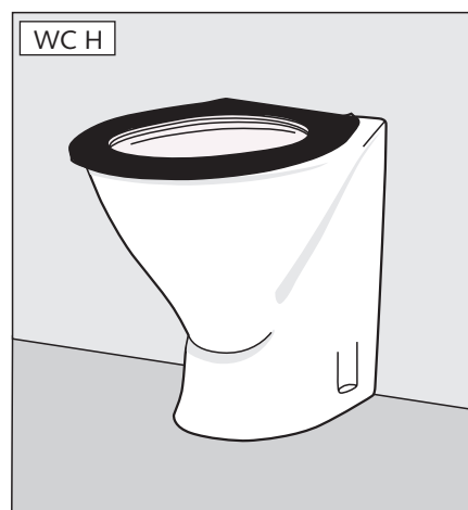
Figure 11 WC for ambulant and semi-ambulant users
