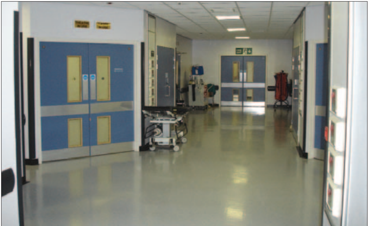
Figure 11 Exit bay with sufficient space to manoeuvre beds and equipment
