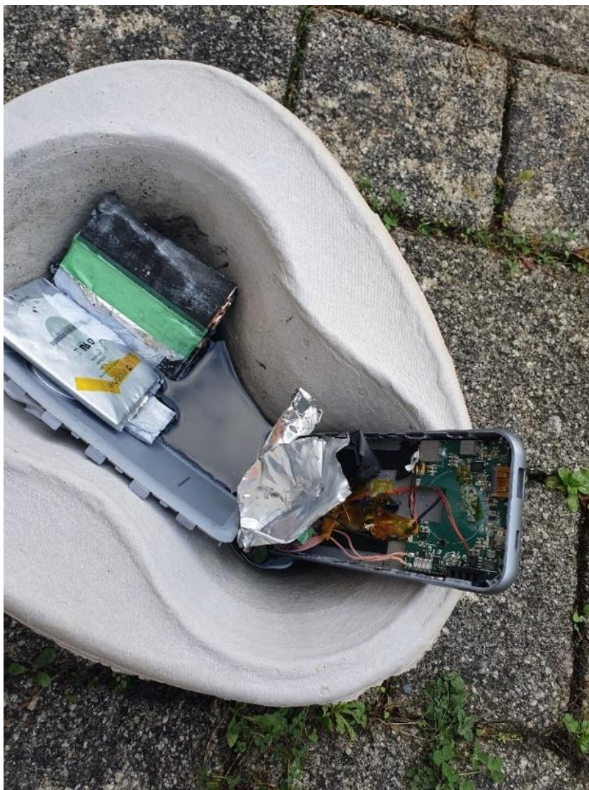
Figure 6 Example of an electrical fire involving a mobile phone battery
