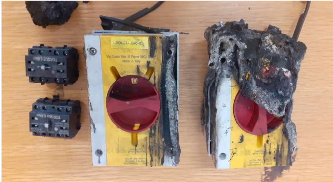
Figure 6 Example of an electrical-related fire attributed to the installation of an inappropriate AC isolator on a Photovoltaic (PV) system.
