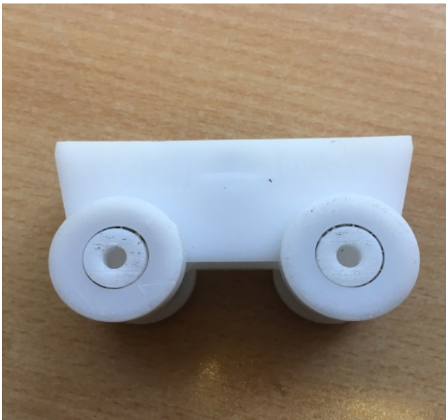
Photo 6 – Complete bracket / roller (without steel bolt and plate)
